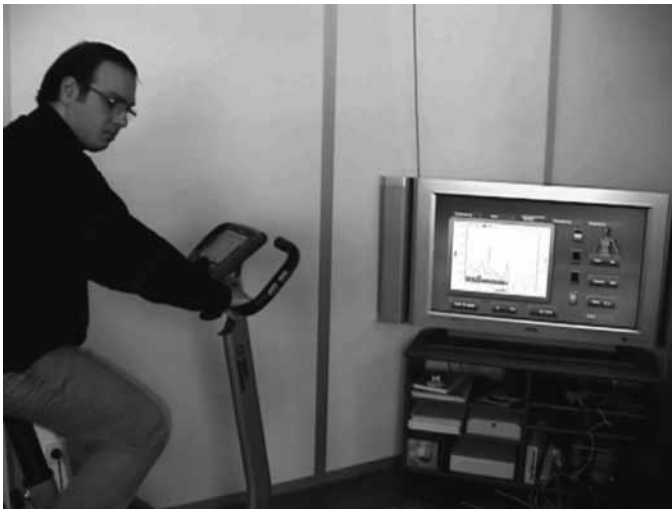
Fig. 3 Evaluation: The volunteer and the ergometer are on the left side, the GUI is shown on a digital TV set, sensors are on the body of the volunteer.
